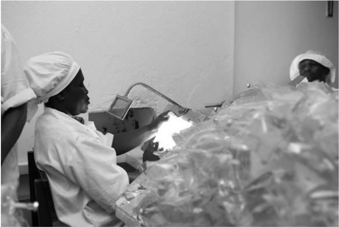
Photo 7: Employees checking each IV bag, one at a time, to ensure there are no unwanted particles in the fluid or damage to the IV bag.
