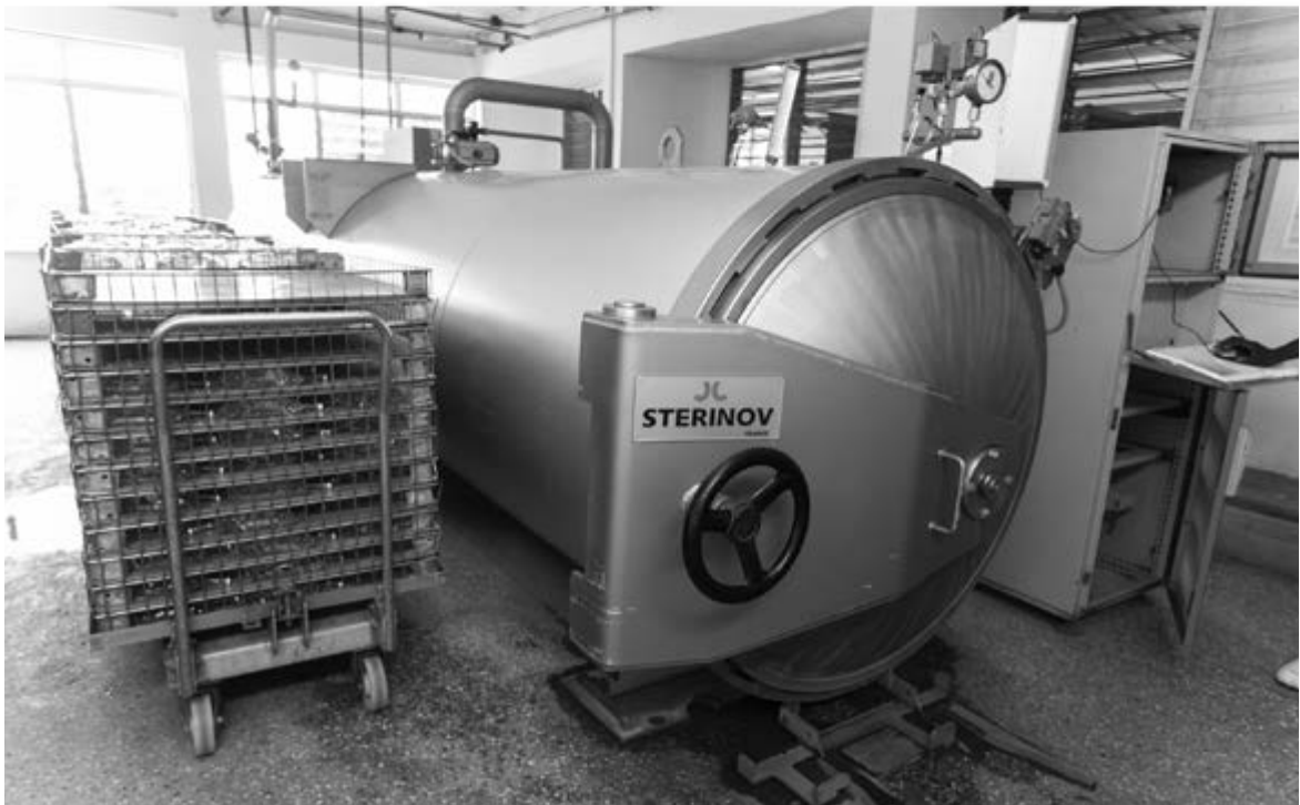
Photo 6: IV fluids about to enter the sterilizing machine. The machine can hold over 2,000 half-litre pouches at a time.
