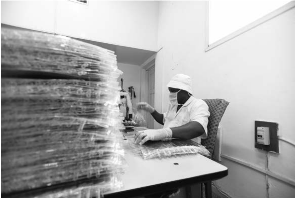
Photo 3: An employee heat stamping the manufacture and expiry date on the IV bags. Each individual does approximately 3,500 to 4,000 bags per day.
